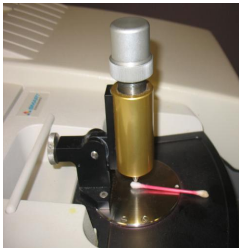
ATR module for experimental FTIR spectra measurements
